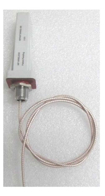
Note: Prototype shown here. The actual antenna will have 10" long cable with straight SMA Male connector.
